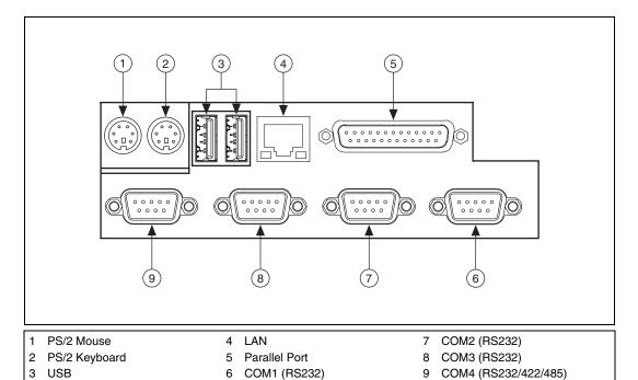
Figure 1-1. I/O Port Arrangement
